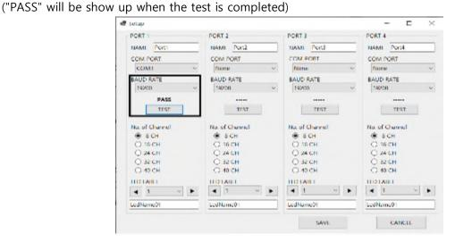
4) When it shows "FAIL", Change the speed of Communication in order from 19200 to 2400(19200  $\rightarrow$  9600  $\rightarrow$  4800  $\rightarrow$  2400) and Test again.
