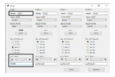
7) Save the setting by pressing Save Button and check if the monitoring program is working normally.
