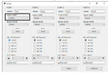
3) Test the Communication between ANS ↔ PC by pressing Test Button.
